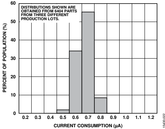
Figure 22. Current Consumption at 25°C, Wake-Up Mode, V_S = 2.5 V
