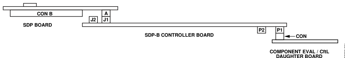
Figure 1. Connecting the SDP Breakout Board
