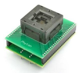
DIP40/BGA48 specialized adapter for FLASH memory. Device package dimensions: 8.0x 6.0 x 1.3 mm, 0.8 mm pitch
