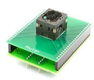
DIP40/BGA48 specialized adapter for FLASH memory. Device package dimensions: 8.15 x 6.15 x 1.0 mm, 0.8 mm pitch.
