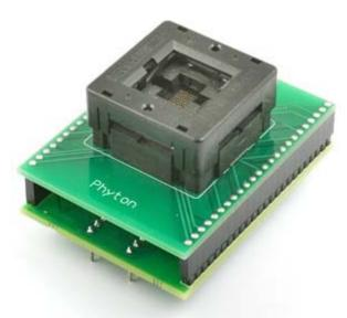
DIP48/BGA48 specialized adapter for FLASH memory. Device package dimensions: 8.0x 6.0 x 1.3 mm, 0.8 mm pitch
