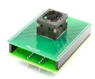
DIP48/BGA48 specialized adapter for FLASH memory. Device package dimensions: 10.0 x 6.0 x 1.0 mm, 0.8 mm pitch
