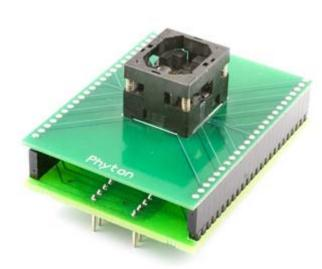
DIP48/BGA48 specialized adapter for FLASH memory. Device package dimensions: 8.15 x 6.15 x 1.0 mm, 0.8 mm pitch
