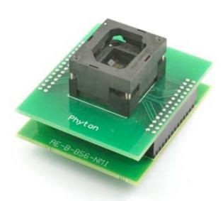
DIP40/BGA56 specialized adapter for FLASH memory. Device package dimensions: 7.7 x 9.0 x 1.0 mm, 0.75 mm pitch.
