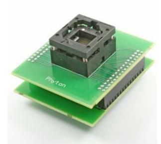
DIP40/BGA64 specialized adapter for FLASH memory. Device package dimensions: 10.0 x 8.0 x 1.2 mm, 1.0 mm pitch.
