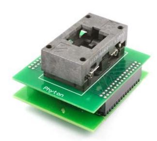
DIP40/BGA64 specialized adapter for FLASH memory. Device package dimensions: 13.0 x 11.0 x 1.4 mm, 1.0 mm pitch.
