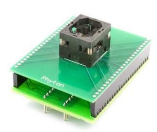
DIP40/BGA64 specialized adapter for FLASH memory. Device package dimensions: 11.6 x 8.0 x 1.2 mm, 0.8 mm pitch.
