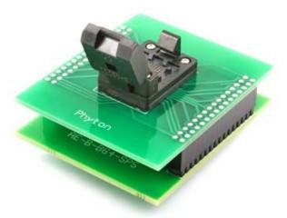
DIP40/BGA64 specialized adapter for FLASH memory. Device package dimensions: 9.0 x 9.0 x 1.4 mm, 1.0 mm pitch.
