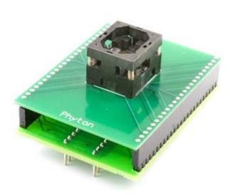
DIP40/BGA84 specialized adapter for FLASH memory. Device package dimensions: 11.6 x 8.0 x 1.0 mm, 0.8 mm pitch.
