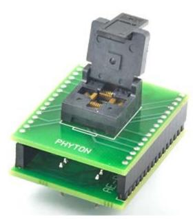
DIP28/MLF28 specialized adapter for Microchip PIC microcontrollers in MLF/QFN packages.
