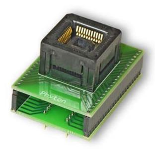
DIP28/PLCC28 universal adapter with open top socket.
