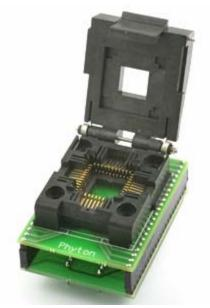
DIP28/PLCC32 specialized adapter for EPROM/FLASH with clam shell socket.
