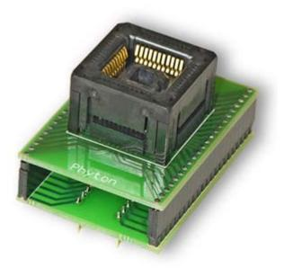
DIP28/PLCC32 specialized adapter for EPROM/FLASH with open top socket.
