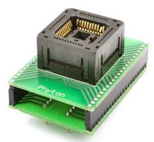
DIP32/PLCC32 specialized adapter for EPROM/FLASH with open top socket.
