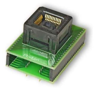
DIP44/PLCC44 universal adapter with open top socket.
