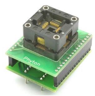
DIP28/QFP32 specialized adapter for Atmel microcontrollers.
