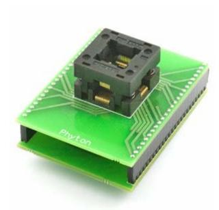
DIP48/QFP48 universal adapter. Device package dimensions: body - 7.0 x 7.0 x 1.5 mm, body with pins - 9.0 x 9.0 mm, 0.5 mm pitch.
