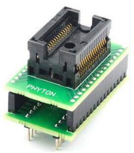
DIP28/SOIC28 universal adapter. Device package dimensions: body width 300 mil (7.65 mm), 1.27 mm pitch.
