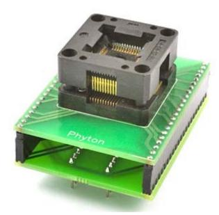
DIP40/QFP44 specialized adapter for microcontrollers. Device package dimensions: body - 10.0 x 10.0 mm, 0.8 mm pitch.
