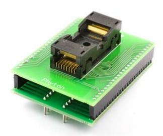
DIP40/TSOP48 specialized adapter. Device package dimensions: 12 x 20 mm, 0.5 mm pitch.
