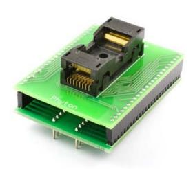
DIP40/TSOP48 specialized adapter for NAND Flash devices. Device package dimensions:12 x 20 mm, 0.5 mm pitch.
