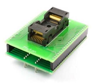
DIP48/TSOP48 universal adapter. Device package dimensions: 12 x 20 mm, 0.5 mm pitch.
