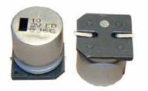
Type AEB capacitors are it for high voltage applications like input bus capacitors in board mounted miniature AC/DC supplies. The AEB's low impedance in ratings up to 450 Vdc, and long life, make it ideal for power supply input and other high voltage applications. The vertical, cylindrical cases make easy automatic mounting and reflow soldering.
