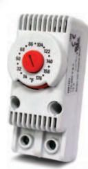
The Heating version (red dial, NC) has closed contacts when the temperature is below the set point value and opens with rising temperature.
