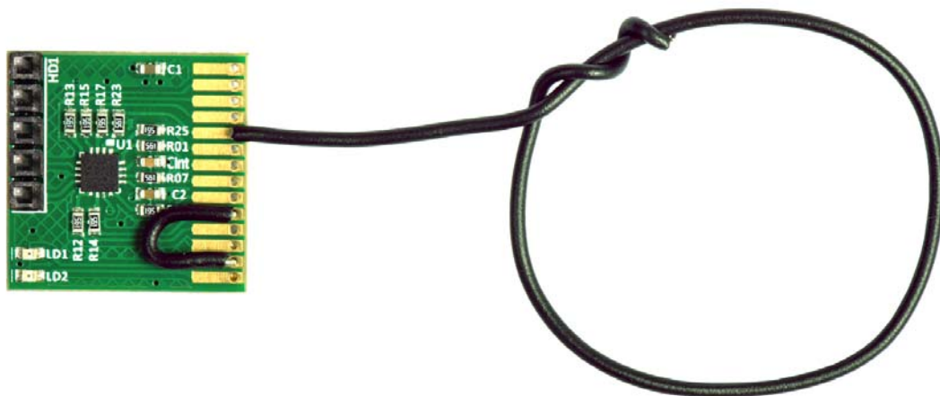
Figure 3-2. A Proximity Sensor Implementation Using a Wire Loop
