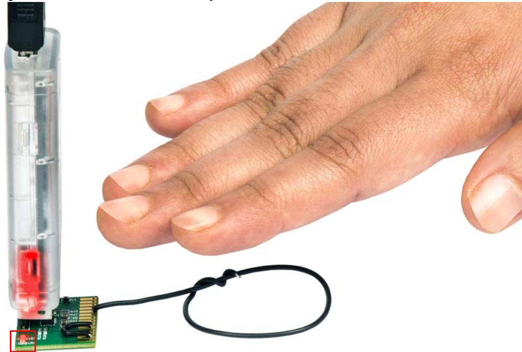
Figure 3-13. LED Glows on Proximity Detection
