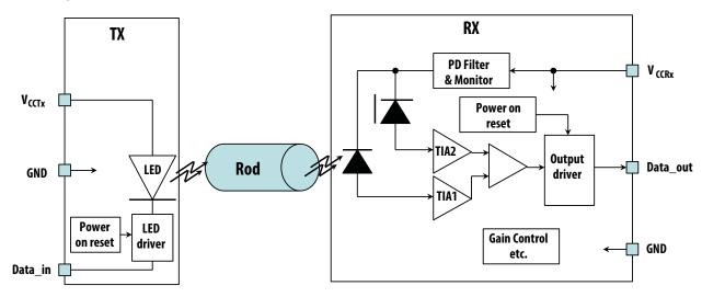
A low Input signal at Data\_in results in a low output signal at Data\_out (non-inverted Tx to non-inverted Rx).
