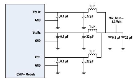
Figure 9. Recommended Power Supply Filter
