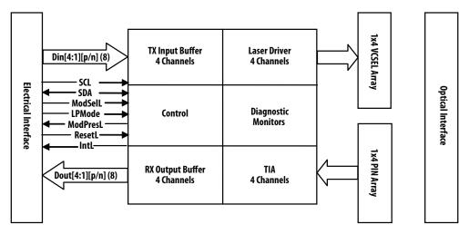
Figure 1. Transceiver Block Diagram
