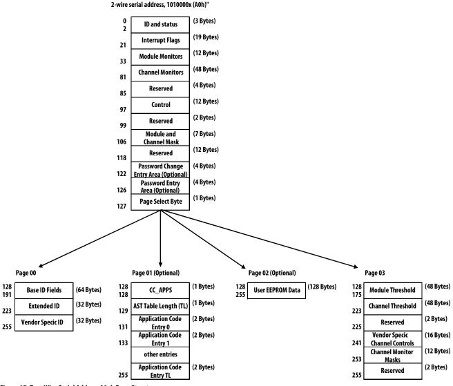
Figure 17. Two-Wire Serial Address A0xh Page Structure
