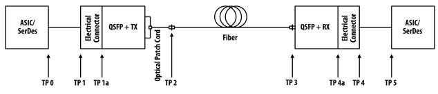
TP0 : Host ASIC transmitter output at ASIC package contact on the Host board
