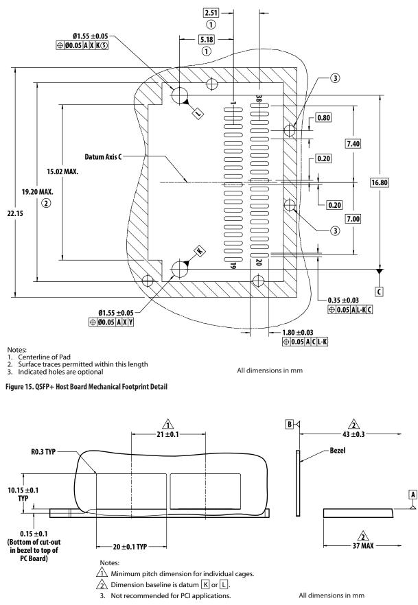
Figure 16. Host Board Bezel Design
