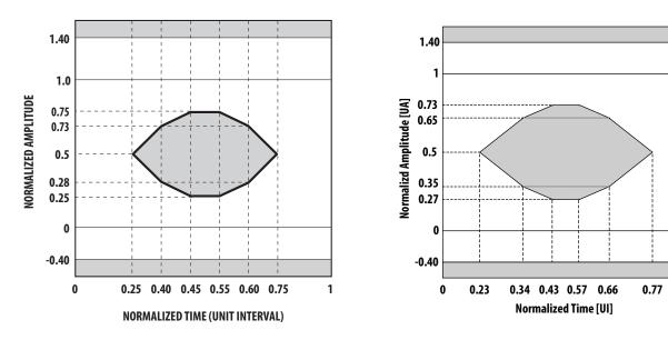
Figure 5a. Transmitter Optical Eye Mask Definition
