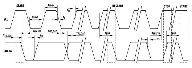
Figure 12. TWS Interface Bus Timing
