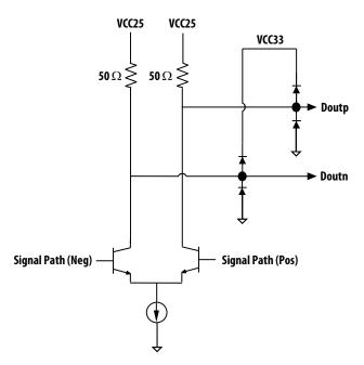
Figure 11. Receiver Data Output Equivalent Circuit
