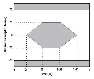
Figure 3. Electrical Eye Mask Coordinates at Hit ratio 5 x 10<sup>-5</sup> hits per sample
