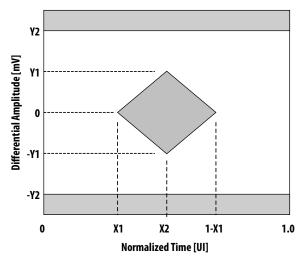
Figure 4. Rx Electrical Eye Mask Coordinates (TP4) at Hit ratio 5 x  $10^{-5}\,$  hits per sample
