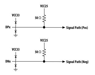
Figure 10. Transmitter Data Input Equivalent Circuit
