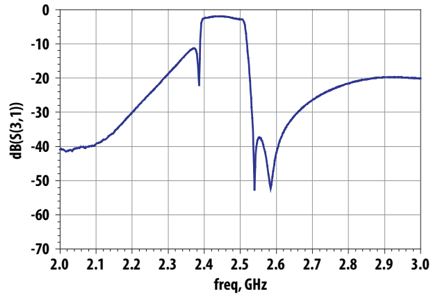
Figure 4. RX Path 2 – 3 GHz Frequency Response
