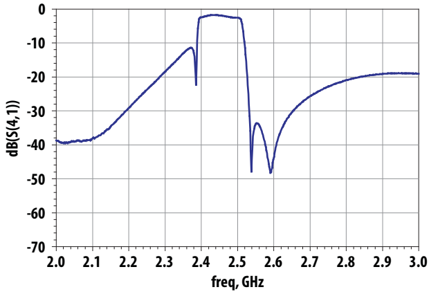
Figure 7. BT Path 2 – 3 GHz Frequency Response
