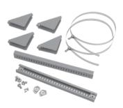
Use to mount CONCEPT  $^{\rm TM}$  , Networking and wall-mount enclosures to poles of various sizes and shapes. Simply attach the plated steel channel bar to the mounting holes at the back of the enclosure and wrap the stainless steel strap around the pole and through the bar. Kit includes two mounting channels, two straps suitable for 3-in. (76-mm) to 12-in. (305-mm) diameter pole and mounting hardware.
