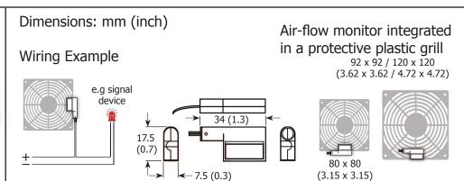
The air-flow monitor provides a simple alternative to indicate positive or negative air flow of fans or blowers. When properly installed and connected in series with an optical (i.e. LED) or audible signaling device, a bi-directional switch will activate an electrical contact if the air flow of the fan falls below 8.2 ft/s, turning the signaling device on or off. The AFM monitor can also be attached to an existing plastic grill or quard.
