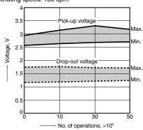
4. Electrical life (1A 30V DC resistive load) Tested sample: AGN2004H, 6 pcs. Operating speed: 20 cpm
