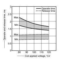
6-(2). Operate and release time (with diode) Tested sample: AGN2004H, 6 pcs.
