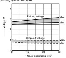
4. Electrical life (1A 30V DC resistive load) Tested sample: AGQ200A4H, 6 pcs. Operating speed: 20 cpm
