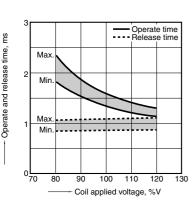
6-(2). Operate and release time (with diode) Tested sample: AGQ2004H, 10 pcs.
