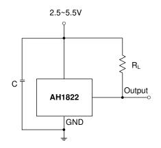
Notes: 4. C is for power stabilization and to strengthen the noise immunity, the recommended capacitance is  $10nF \sim 100nF$ . R<sub>L</sub> is the pull-up resistor, the recommended resistance is  $10K\Omega \sim 100K\Omega$ .
