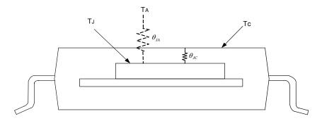
Notes: 2.  $\theta_{JA}$  should be confirmed with heat sink thermal resistance. If there is no heat sink contact,  $\theta_{JA}$  will almost be the same as  $\theta_{JC}$ ..
