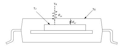
Notes: 5.  $\theta_{JA}$  should be confirmed with what heat sink thermal resistance. If no heat sink contacting,  $\theta_{JA}$  is almost the same as  $\theta_{JC}$ .
