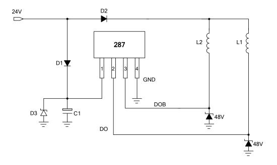
Note: The optional Capacitor C1 and Diode D3 are for power stabilization. C1 is recommended to be E-Cap., luF/25V; D3 is recommended to be Zener Diode,  $V_Z$ =27V. Which C1and D3 value need to be fine tuned to optimize design for different coils and power suppliers.
