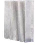
All testing and power characteristics are based on a vertically mounted orientation. Horizontal mounting is acceptable with fins in the upward position with approximately 20% degradation in performance.
