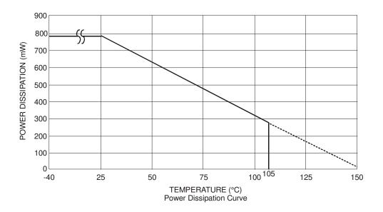
Notes: 10. U-DFN2020C-6 exposed pad soldered to minimum recommended landing pads (see Package Outline Dimension section) on a two-layer 2oz. copper FR4 PCB (1.6mm thickness) with no thermal vias in exposed PADs or any copper flood connecting to the landing pattern of the exposed pad.
