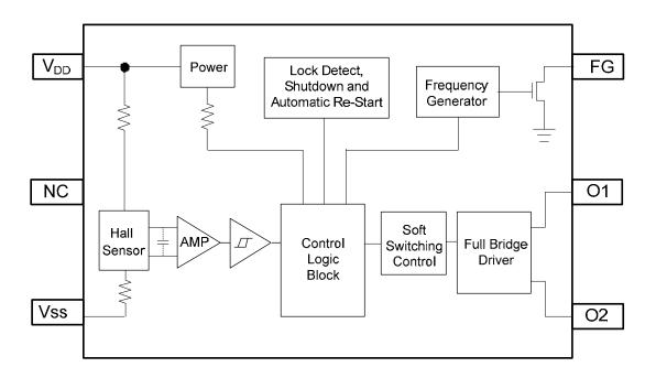
Notes: 2. The AH5794 has an open-drain tachometer FG output that follows the magnetic change frequency. Typically a pull-up resistor of  $10k\Omega$  is recommended from FG pin to the supply voltage.
