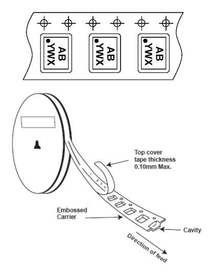
Notes: 14. The taping orientation of the other package type can be found on our website at http://www.diodes.com/datasheets/ap02007.pdf.
