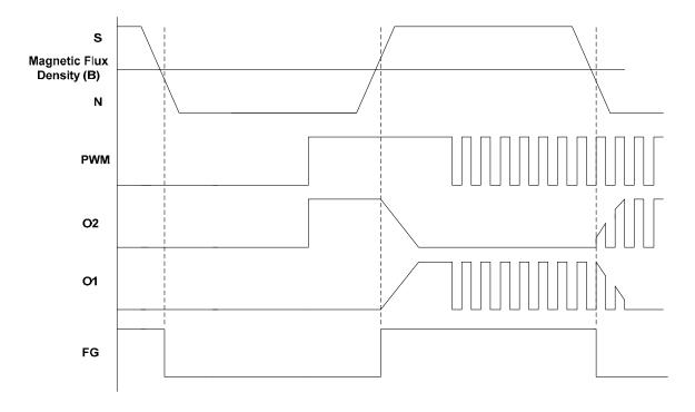
Frequency of PWM speed control signal can be between 15Hz to 50kHz. Recommended typical PWM signal frequency is 25kHz to keep switching frequency away from audible band. If PWM signal level at PWM pin stays low for longer than 65ms typical, the outputs are disabled.
