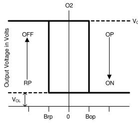
Magnetic Flux Density in Gauss
