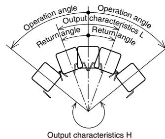
2) Output ( $V_o$ ) characteristics (The sphere must be stationary.)
