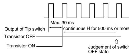
2) The switch should be mounted keeping away from the vibration generator such as motor. Fix the PC board firmly in order to prevent resonance with the vibration generator, or the contact chattering of a switch may occur by the movement of a
