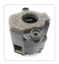
An integrated, low-noise fan draws a greater volume of cabin air across the temperature sensor, providing a faster response as compared to traditional passive sensors. This can result in a more accurate climate control, leading to better cabin comfort. This sensor can also help improve the efficiency of the temperature control system by reducing the on / off cycles of the heating and cooling system.
