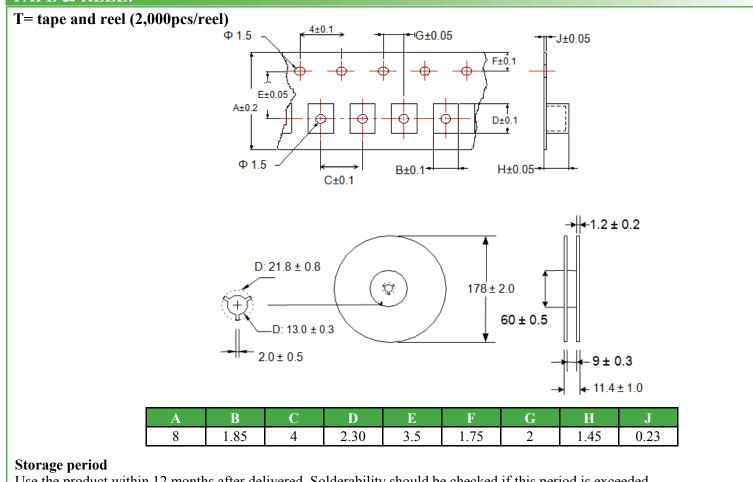
Use the product within 12 months after delivered. Solderability should be checked if this period is exceeded. **Dimension: mm**
