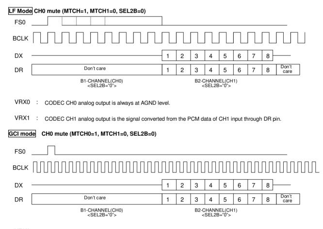
VRX0 : CODEC CH0 analog output is always at AGND level.
