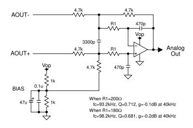
Figure 10. External 2<sup>nd</sup> order LPF Circuit Example (using op-amp with single power supply)
