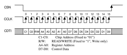
Figure 8. Control I/F Timing
