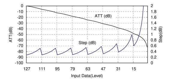
Figure 10. ATT characteristics
