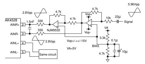
Input RC filter response : fc = 160kHz, g = -0.07dB at 20kHz, -0.26dB at 40kHz.
