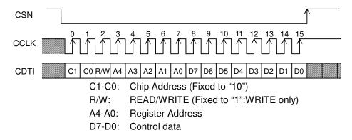
Figure 9. Control I/F Timing
