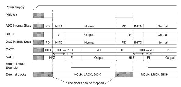
• INITA: Initializing period of ADC analog section (516/fs).
