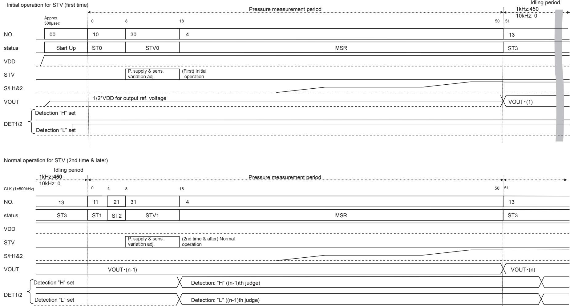
**Description of Operation Timing Status (pressure detection circuit effective)**
