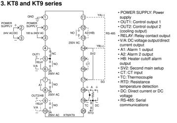
Note: That main setting No. 2 will not be possible on the KT8 and KT9 when the communications functions is added.
