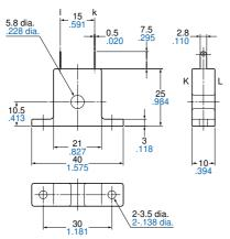
Note: CT1 or CT2 for current detection is provided as an accessory when heater burn-out alarm function is added.
